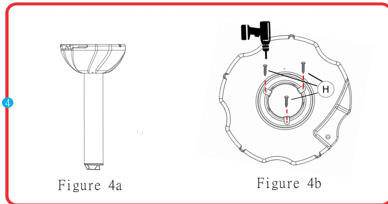
Turn Base Assembly (A) upside down (Figure 4a), and use 3 Self Tapping Screws (H) to secure brackets on bottom of column to the reservoir as shown in Figure 4b. Feed female quick connect end of Hose (D) through the bottom of the Base Assembly (A).
