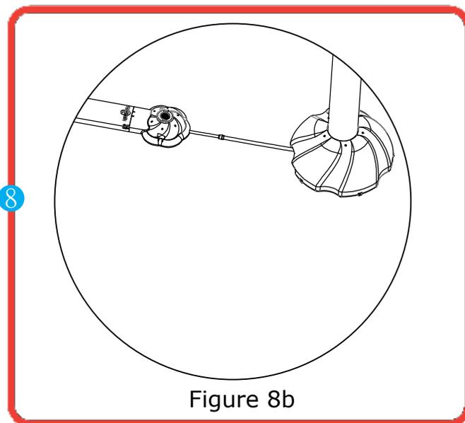
Connect Cannon Blaster hose directly to garden hose (Figure 8a) or to Aqua-Station adapter (Figure 8b)
