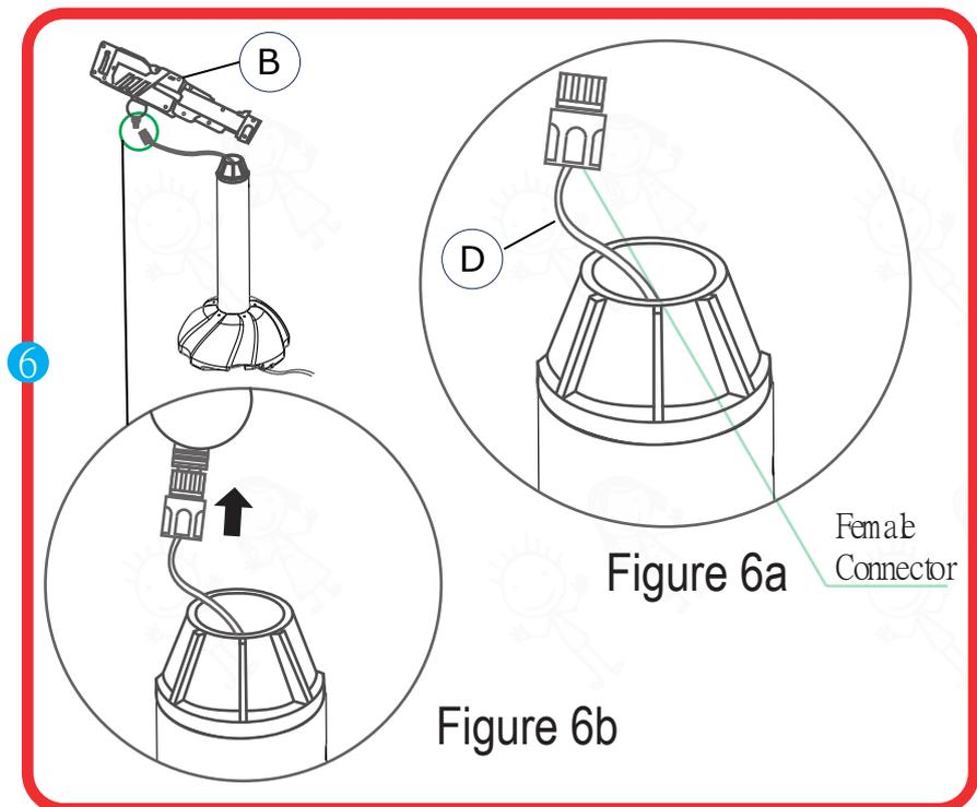
6 Pull the female end of Hose (D) with the quick connector up through the column (Figure 6a), and push it firmly onto the Cannon (B) fitting until it clicks into place (Figure 6b).
