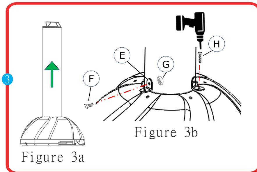
Pull up the column and remove the bubble wrap around it. Holding the column in the upper most position, attach 3 Brackets (E) to column using Machine Screws (F), and Lock Nuts (G) as shown in Figure 3b. Rotate column to align Brackets (E) as desired and secure to base using 3 Self Tapping Screws (H). Do not use holes on base to secure Brackets (E).
