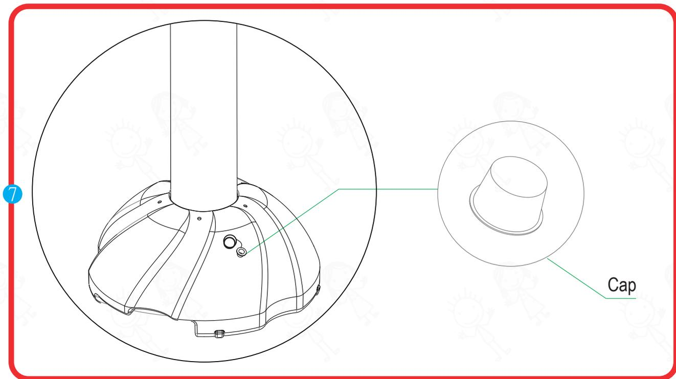
7 Remove the cap and fill the base with water.
